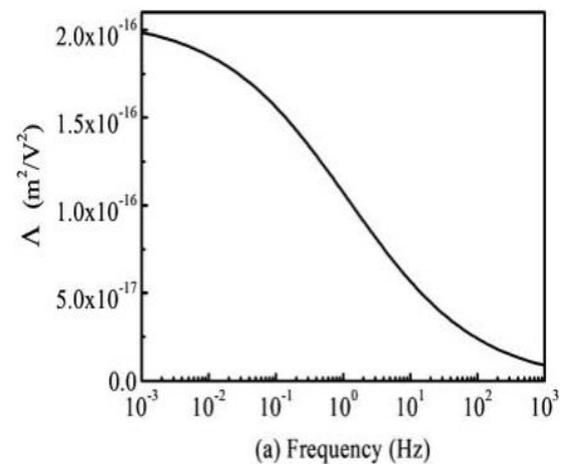
**Figure No. 8:** Actuation factor as a function of frequency at 35°C.
