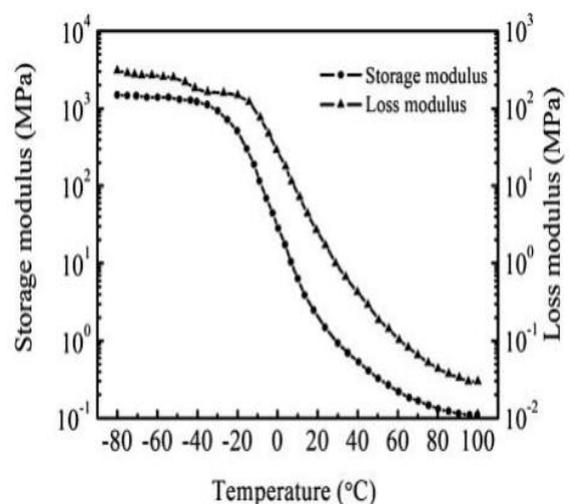
**Figure No. 4:** Storage and loss moduli as a function of temperature at a frequency of 0.1 Hz.
