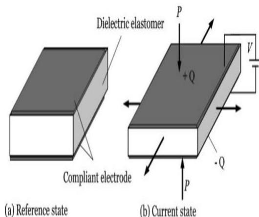
**Figure No. 2:** Actuation of the dielectric elastomer
