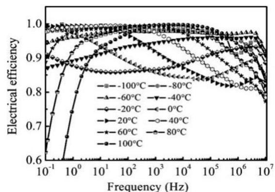
**Figure No. 6:** Electrical efficiency of the VHB 4910 at different temperatures.
