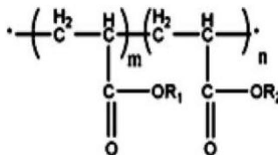
**Figure No. 1:** Commercial trade secrets related to the chemical composition of VHB 4910 acrylic elastomer with  $m$ ,  $n$ , and  $R_2$ .
