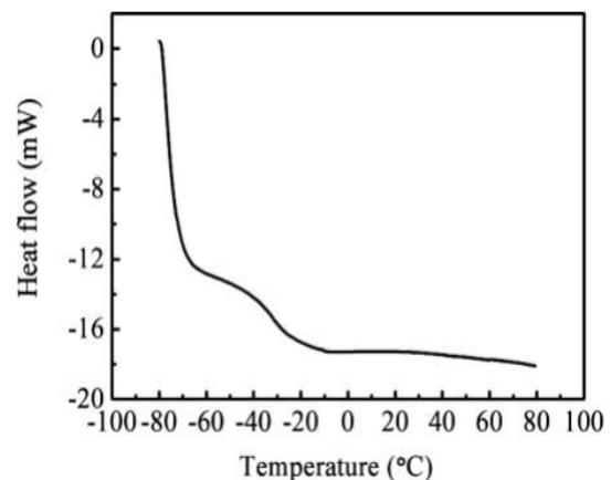
**Figure No. 3:** DSC thermogram of the VHB 4910
