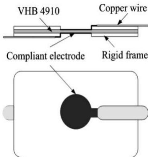
**Figure No. 7:** Configuration of the specimen used for electromechanical experiments.
