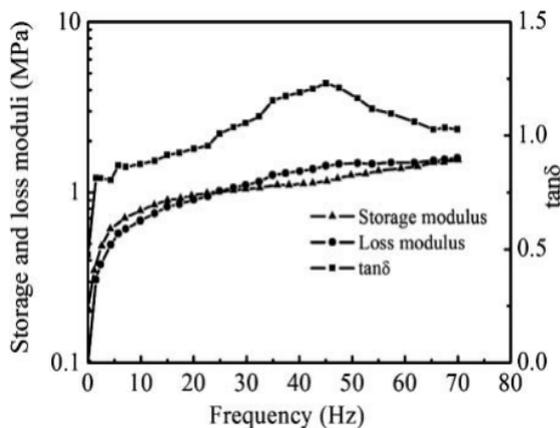
**Figure No. 5:** Frequency dependence of loss factor, storage, and loss moduli at 35°C.
